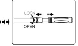
Turn the ring in anti clockwise until feel it stop, adjust the length of alu pole you want, then turn the ring in clockwise to
