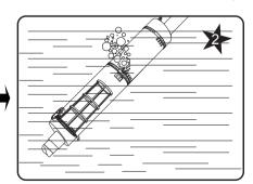
3. Place the motorized head of cleaner into the spa/pool which more than 38cm water,it can start-up automatically.
