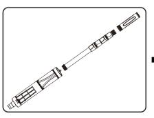
1. Assemble the handle with small end of the pole, main body with the other end.
